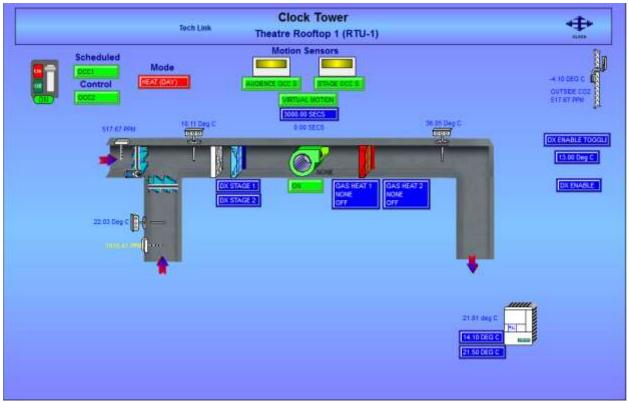
Figure 8: DDC Image of RTU-1
